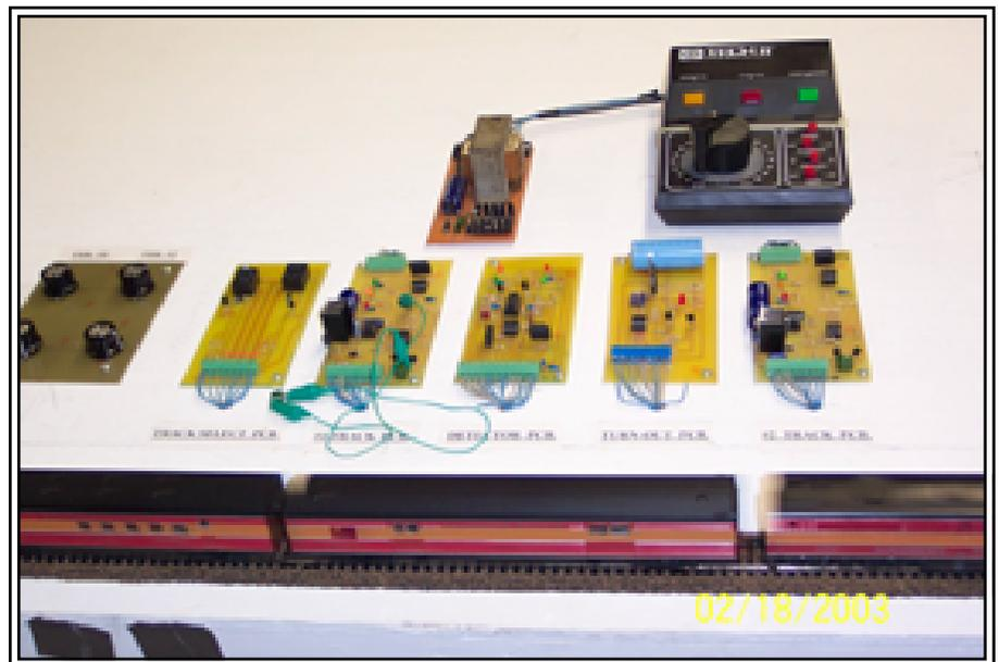
The electronic circuits; Detector, Throttles, Switching/Control, five and twelve volt power supplies.
