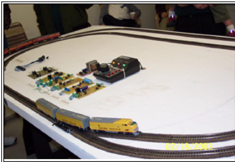
The trains run around and around on their own loop sharing a common section of track while the electronic control monitors them, switches them into and out of the common section and controls the throttles so they never collide.
