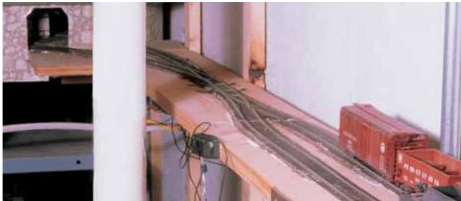
▲ The Pennsylvania RR tracks at Sciotovale form two legs of a wye with the Maumees main line as its base. This allows the Pennsy steam engine to be turned around before it runs back into staging.
