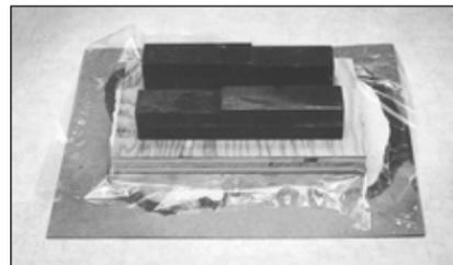
**Fig. 11 ADD WEIGHT.** Place a scrap of plywood or hardboard on top of the plastic wrap, then add a little weight.
