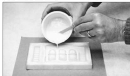
**Fig. 8 POURING PLASTER.** Add stripwood for the horizontal sash pieces through the window centers, then carefully pour the Hydrocal.
