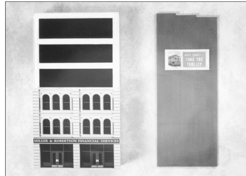
**Fig. 15 STRUCTURE FRAME.** The frame is 1 x 3 lumber with a Masonite hardboard back. Once the Plexiglas is in place, casting subassemblies can be attached, working upward from the ground floor. The thin side panel will be cemented to the right side of the frame later.
