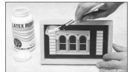
**Fig. 3 STARTING THE MOLD.** Begin making the mold by applying several thin coats of liquid latex with an inexpensive paintbrush. Be sure to eliminate any air bubbles.
