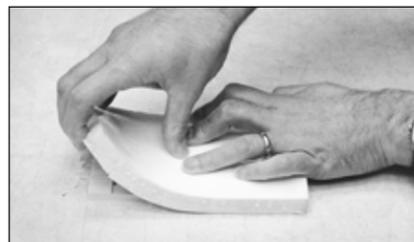
**Fig. 12 REMOVING CASTING.** Press the rear of the casting on a smooth surface and carefully peel the mold away from the casting.
