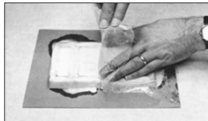
**Fig. 10 PLASTIC BACK.** Give the casting a flat back by applying a piece of plastic wrap. Don't trap any air bubbles under the plastic.
