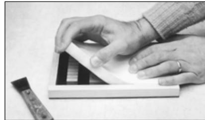
**Fig. 7 REMOVING THE MOLD.** After the sealant has cured, carefully peel the mold away from its pattern.
