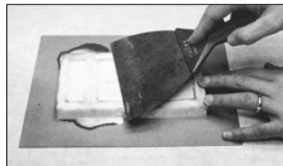
**Fig. 9 SMOOTH PLASTER.** Slightly overfill the mold, then remove the excess Hydrocal with the drywall spatula.
